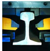
Clamping system in starting position
