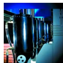
Clamping cylinders each with 1000 kN clamping force
