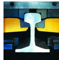
Rail in welding position
